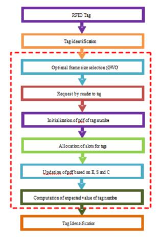
Fig. 1. Proposed Tag Anti Collision Method Using BEDFSA
