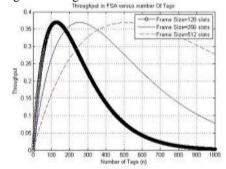
Fig. 2. FSA Throughput For Different Frame Size
